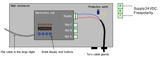
Bring the supply voltage to the connector indicated in the picture. A pre-fuse is not necessary, but if one is used, it should be at least 2 AT. The protective earth is not required for electrical safety, but will protect from EMI fields.
