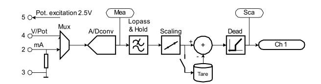
The microcontroller sets the multiplexer "Mux" to measure the V or mA input according to the configuration settings. The input is measured using a 24-bit analog-to-
