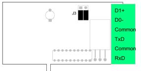
The serial communications card 2000-RS works most often with the factory set jumpers: no termination. But if the RS-485 bus is long (>50 m), the last device on the bus should be terminated.
