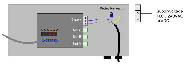
Bring the Live and Neutral wires to the electronics unit as in picture. Connect the Protective Earth wire to the M4 screw using the Faston connector provided - a Faston crimping tool is needed. A pre-fuse is not necessary, but if one is used, it should be at least 500mAT.
