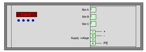
The power supply is brought to the lowest connector terminals 1 and 2. The polarity does not matter. The enclosure may be earthed using the terminal 4.
