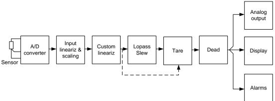
The input signal or sensor is measured with an analog-to-digital converter and other circuitry. A new reading is obtained 3 to 4 times per second. The input circuitry is galvanically isolated from the analog output.
