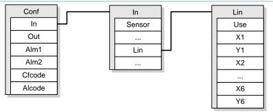
The Lin submenu is used for custom linearization of the input. To enable the linearization, set Use=Yes.
