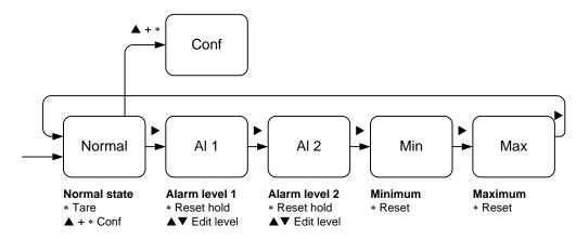
When an alarm LED is blinking, the alarm level can be changed. Press  $\blacktriangle$  or  $\triangledown$  until the first digit starts blinking, then edit as described in chapter Editing.
