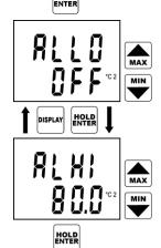
Then you are offered to set alarm of other input value (here temperature of channel 2). The procedure is the same as the above temperature limit setting. Alarm activation of each value can be disabled by setting lower alarm limit of the desired value up to its maximum. This is indicated by OFF reading at the position of numeric value. Value of upper limit of the same alarm is indifferent.
