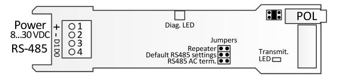
FT20 serial module has a 4-pin terminal block for power supply and RS-485 connection. Serial module features also a round 3.5 mm POL programming connector jack found on many other Nokeval products as well. FT20 radio module contains BNC type antenna connector.
