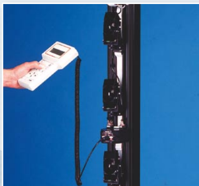
Parameterization using TM1711 Terminal
