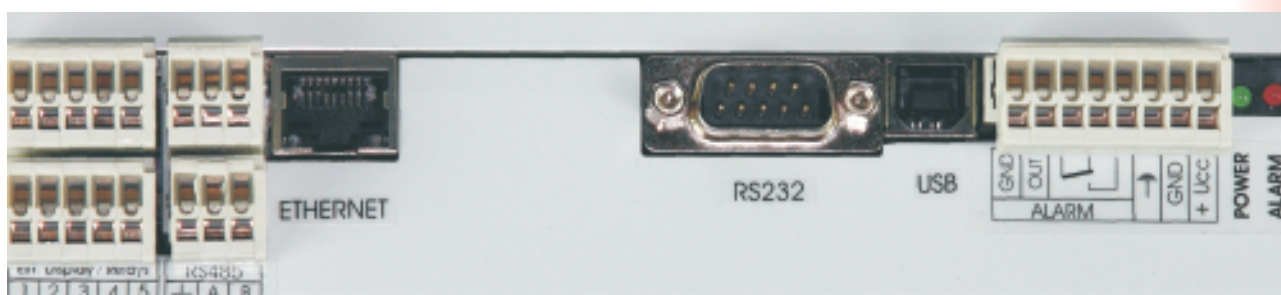
Figure: communication interface, alarm outputs, connection of power - Ethernet interface is optional
