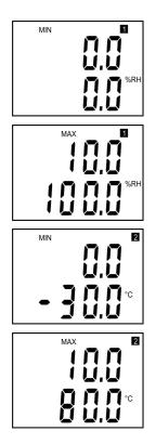
Range and type of value for output 1 (Uout 1 =symbol "1"on display). Type of value, assigned to output 1, is indicated by displayed unit (here %RH = relative humidity). Upper line displays voltage value corresponding to measured value (lower line).
