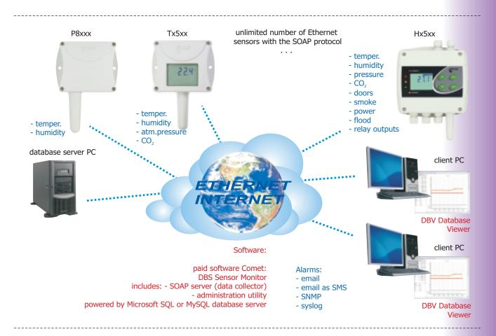
Database program DBS Sensor Monitor for online data acquisition and analysis from Comet sensors is a client-server data acquisition system.
